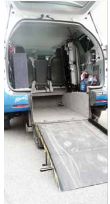
Figure 1: A Toyota Sienna converted to a Wheelchair Accessible Taxi (Victoria)
